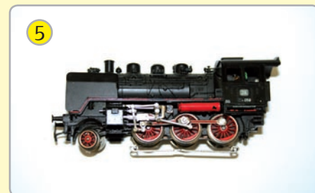
To finish the conversion you only need to re-assemble the body of the loco und make sure that none of the cables gets clamped.
